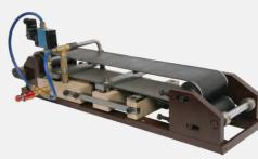
**Belt Guide**For feeding flimsy material & material below 0.1mm
