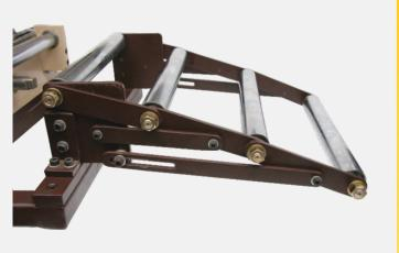
Adjustable Cascade Rolls for smooth material flow at feeder inlet
