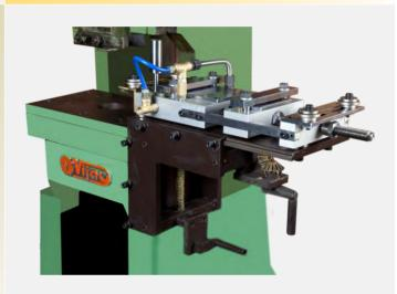
Feeder with Universal Mounting Stand with x-y movement to clamp feeder on press & progressive tooling
