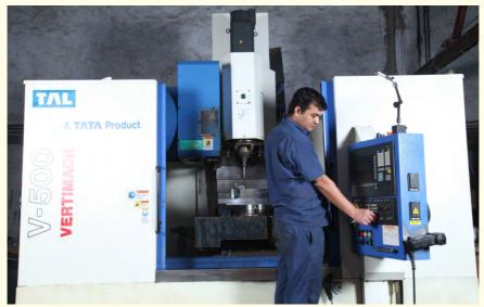
TAL 5-AXIS Vertical Machine Center with RENISHAW Work Piece Off Setting Device & RENISHAW Tool Setter
