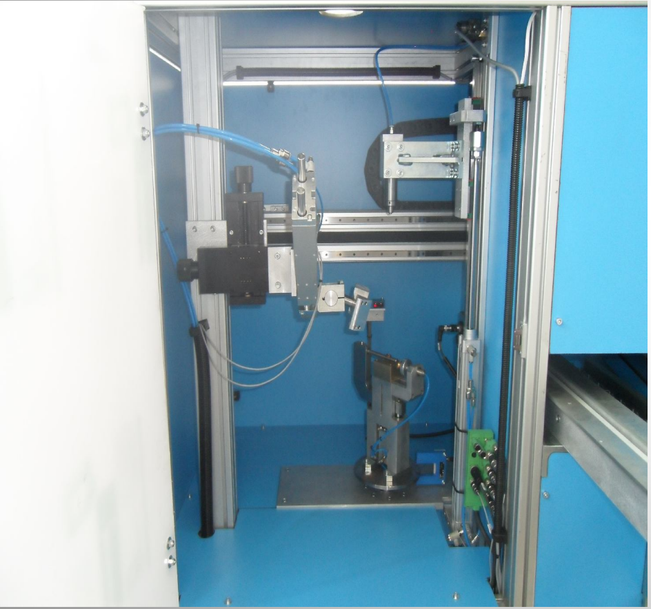
Automatic welding machine for water collectors (GTAW)
