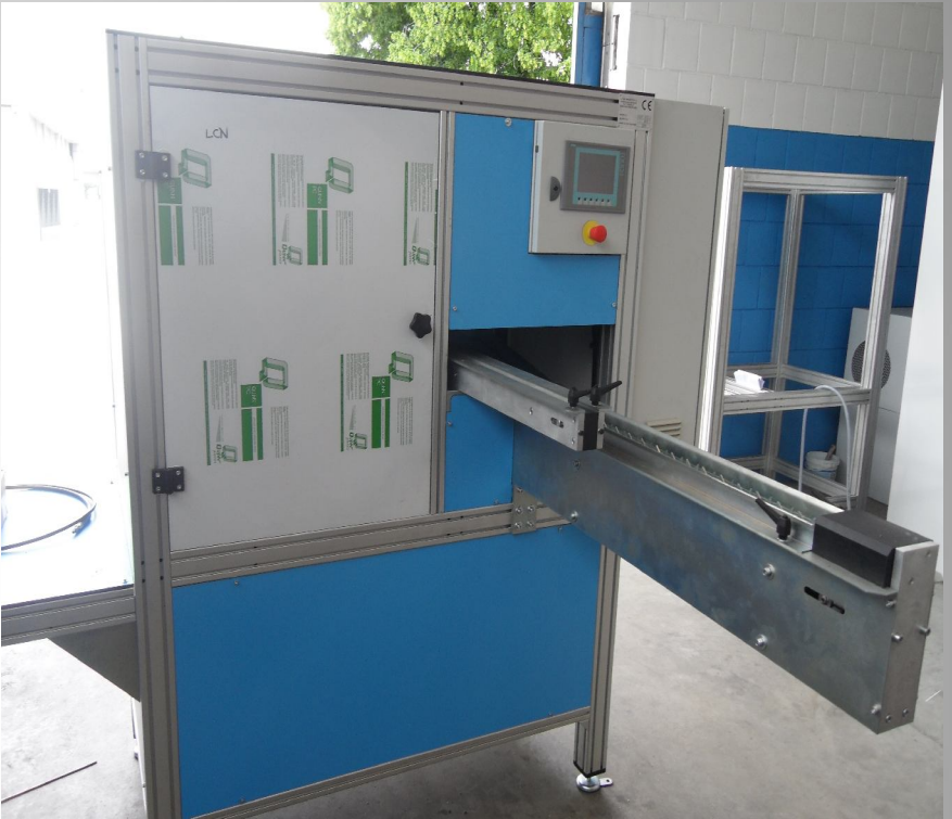
Automatic welding machine for water collectors (GTAW)
