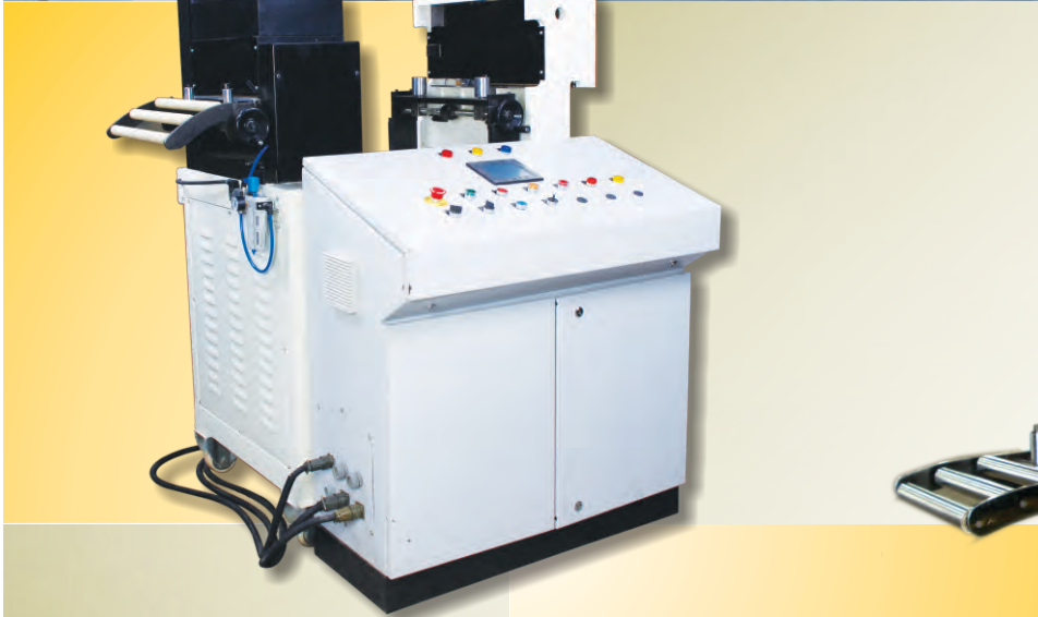
Transformer Lamination Punching, Notching & Variable Cut to Length Line
