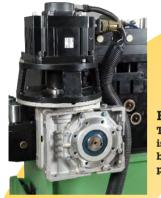
Better Accuracy The Straightener Feeder is Motorised through one brushless servo motor & precision gear box.
